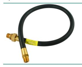
1/2" nominal size hose incorporating a union fitting. This hose does not conform to BS 669 as it does not incorporate a quick disconnect fitting, and therefore should not be used to connect domestic gas appliances in the UK.
